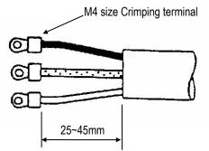
Figure 5.6 Terminal Treatment of Power Cable, Current Output Cable and Digital I/O cable
